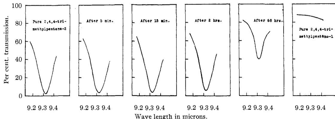
Fig. 1b.—The isomerization of 2,4,4-trimethyl-2-pentene to 2,4,4-trimethyl-1-pentene upon contact with silica gel at room temperature as evidenced by the decrease in intensity of the 9.3  $\mu$  absorption band of 2,4,4-trimethyl-2-pentene.
