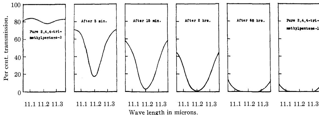
Fig. 1a.—The isomerization of 2,4,4-trimethyl-2-pentene to 2,4,4-trimethyl-1-pentene upon contact with silica gel at room temperature as evidenced by the increase in intensity of the 11.2  $\mu$  absorption band of 2,4,4-trimethyl-1-pentene.
